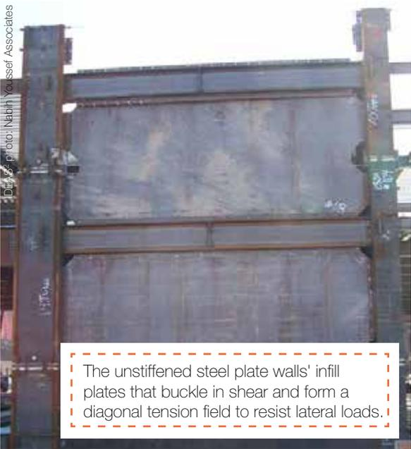
The unstiffened steel plate walls' infill plates that buckle in shear and form a diagonal tension field to resist lateral loads.
