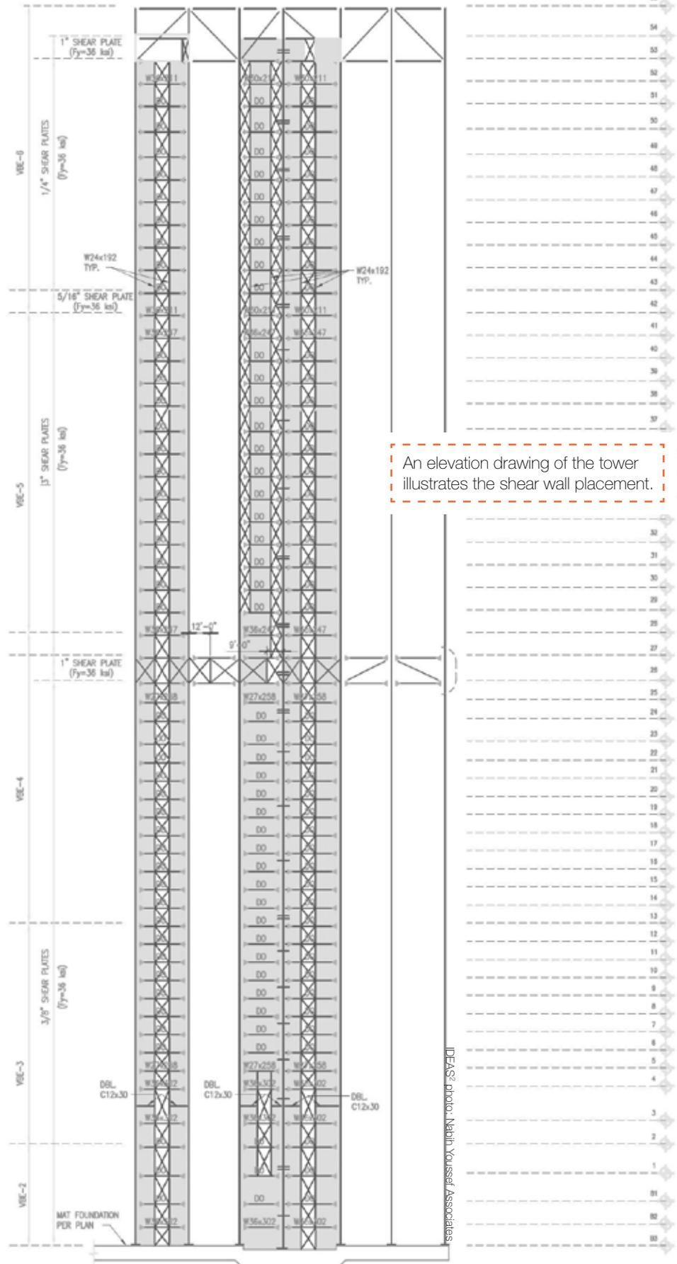
An elevation drawing of the tower illustrates the shear wall placement.
