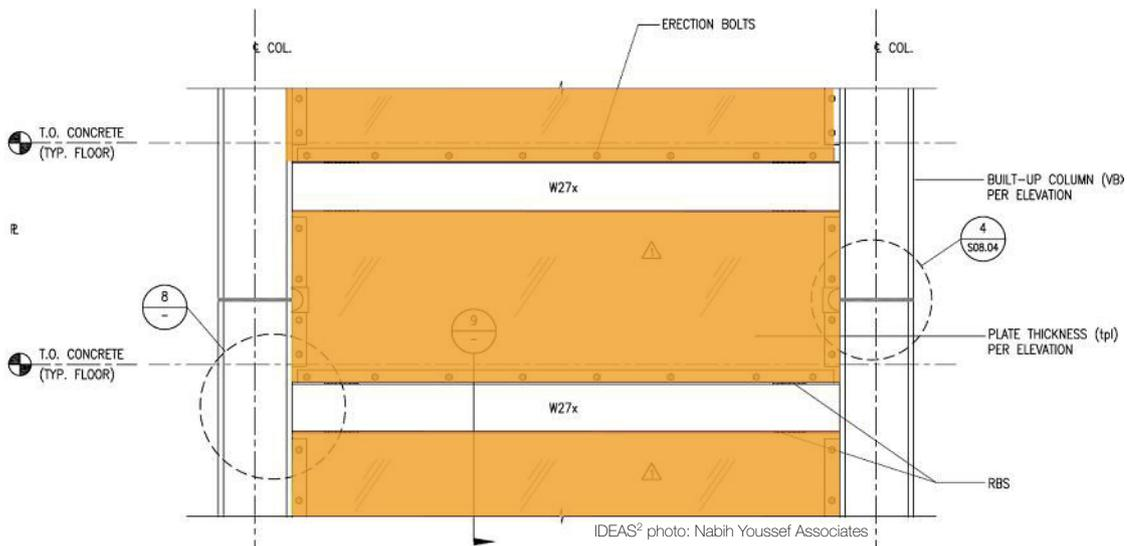
A typical steel plate elevation drawing. The steel plate shear walls resist lateral loads and are designed to “tune” the stiffness of the T-shaped building’s separate wings.
